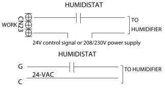
To connect a humidifier, utilize the passive signal "WORK" output (CN23) port as well as the G and C wires on the controller, and wire the humidistat and humidifier per above wiring diagram. When the fan is running, the CN23 relay will be closed, which will allow power to the humidifier when the humidistat is below humidity setpoint. If the thermostat or zone controller has an HUM interface, connect the humidifier directly to the HUM and C ports.
